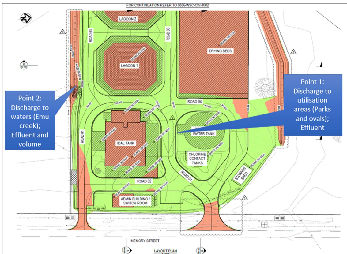
Figure 1 – Grenfell Wastewater Treatment Plan Site Plan
